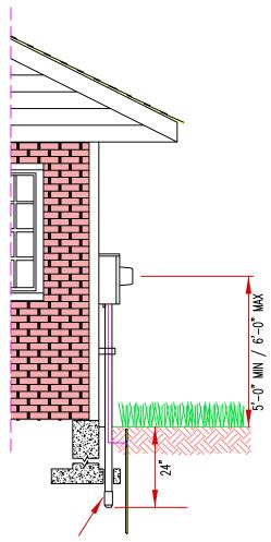
PROTECTIVE BUSHING REQUIRED ON END OF CONDUIT UNLESS COMPLETE CONDUIT SYSTEM IS USED. CONDUIT SHOULD BE STUBBED BELOW CONCRETE FOOTINGS.
